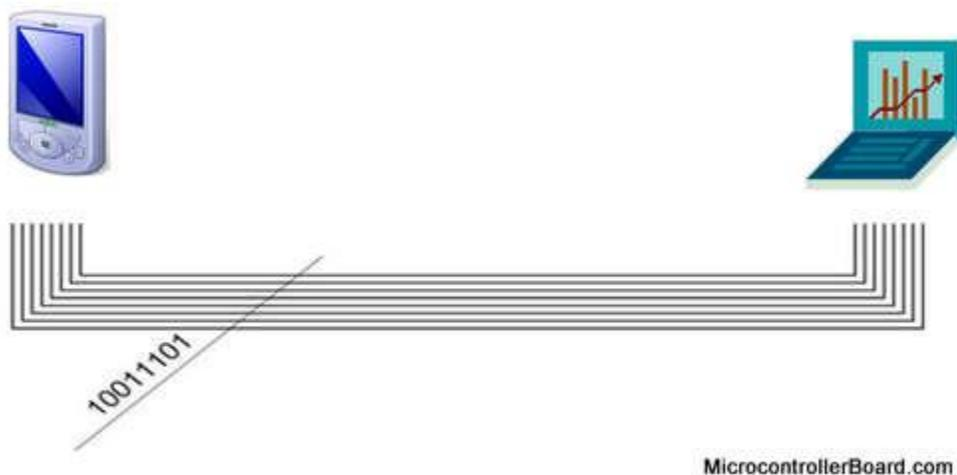
In **data transmission**, **parallel communication** is a method of conveying multiple binary digits (**bits**) simultaneously. It contrasts with **serial communication**, which conveys only a single bit at a time; this distinction is one way of characterizing a communications link.
