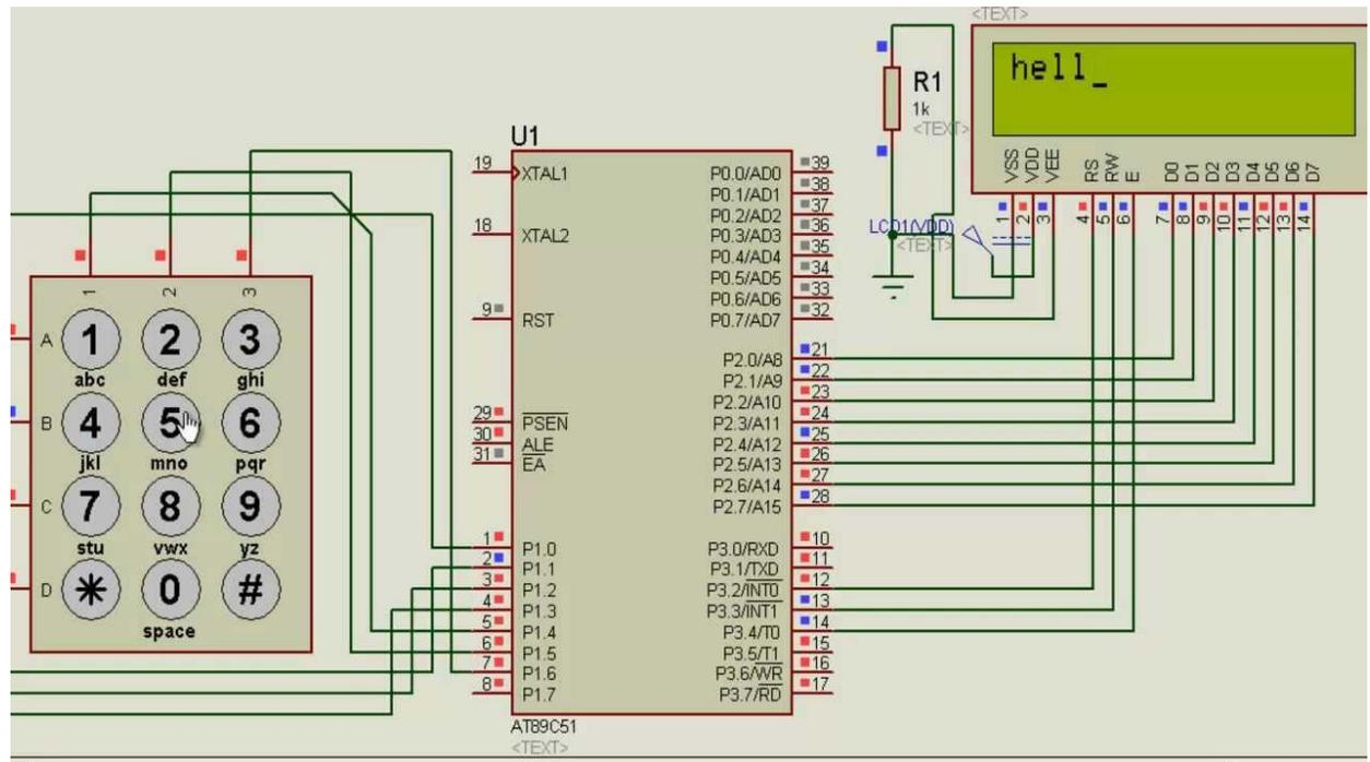
Interfacing is one of the important concepts in microcontroller 8051 because the microcontroller is a CPU that can perform some operation on a data and gives the output. However to perform the operation we need an input device to enter the data and in turn output device displays the results of the operation. Here we are using keyboard and LCD display as input and output devices along with the microcontroller.
